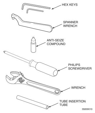
Figure 7-2. Probe Disassembly Kit
